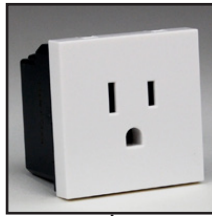
76143X45 North America & Japan NEMA 5-15 Outlet 15 Amp 125V 45x45mm. Duplex Version 76143X45D 45x67.5mm.
