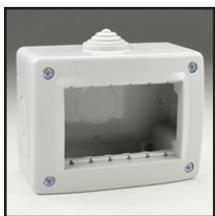
680603X45 Surface Mount Box. 67.5mmx45mm Opening. Gray. Accepts 22.5mm, 45mm & 67.5mmx45mm Devices.
